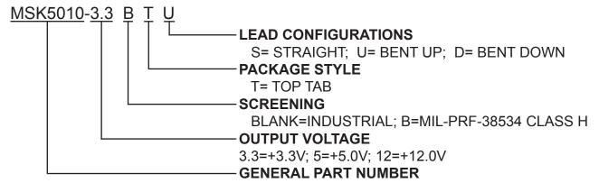
THE ABOVE EXAMPLE IS A +3.3V, MILITARY REGULATOR USING THE TOP TAB PACKAGE WITH LEADS BENT UP.
