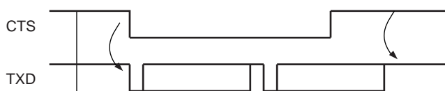
Figure 33-17. Transmitter Behavior when Operating with Hardware Handshaking
