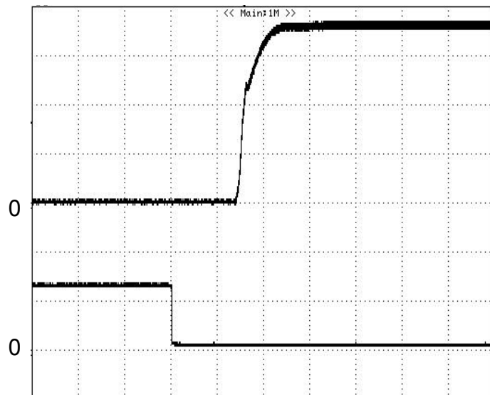
Figure 5: Turn-on transient at zero load current (2 ms/div). Vin=48V Top Trace: Vout, 0.5V/div; Bottom Trace: ON/OFF input, 5V/div
