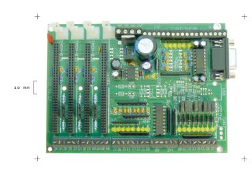
INFO The BB-301S baseboard is designed for the TMCM-301 or TMCM-341 stepper controller to operate with up to three TMCM-035 power drivers in a 24V industrial environment. It provides a small and cost effective solution for a motion control application for up to three size 57 mm stepper motors.
