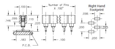
Interconnect Socket Surface Mount Socket Accepts .015"- .025" (0,38 - 0,635 mm) dia leads Single Row Surface Mount Plating Code: Shell Plating: 200 μ" Tin/Lead(93/7) over 100 μ" Nickel Inner Contact Plating: 10 µ" Gold over 50 µ" Nickel
