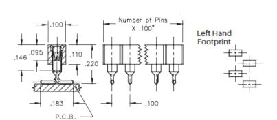
**Description:** Interconnect Socket Surface Mount Socket Accepts .015" - .025" (0,38 - 0,635 mm) dia leads Single Row Surface Mount **Plating Code:** Shell Plating:
