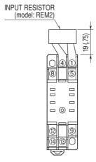
Input shunt resistor attached for current input.
