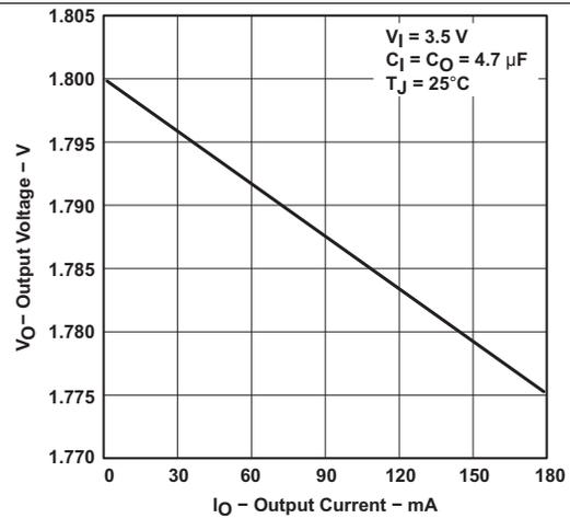
Figure 2. TPS76318 Output Voltage vs Output Current
