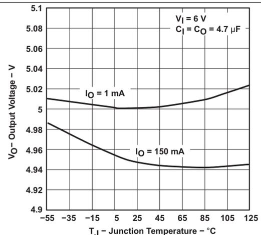
Figure 6. TPS76350 Output Voltage vs Free-Air Temperature
