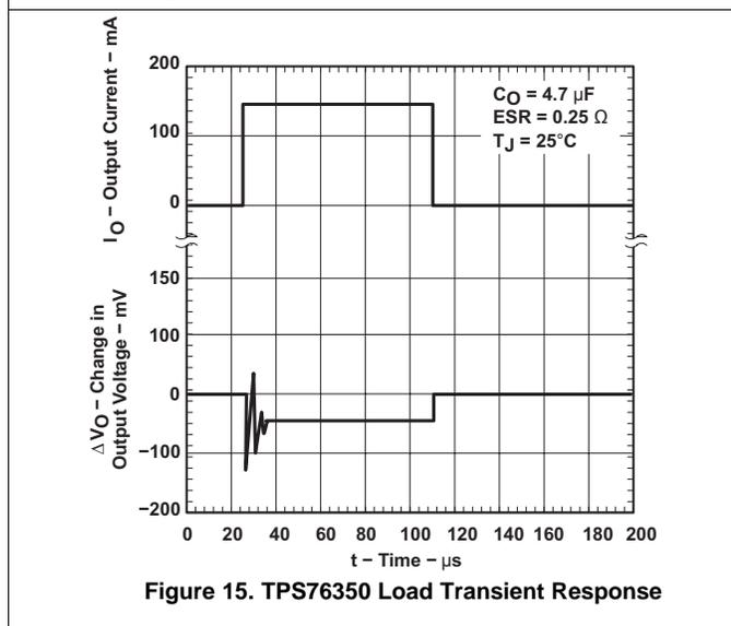
Figure 15. TPS76350 Load Transient Response
