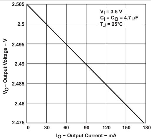
Figure 1. TPS76325 Output Voltage vs Output Current
