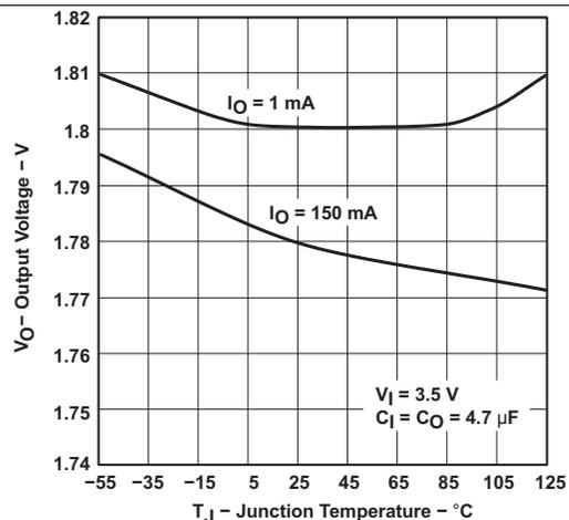
Figure 5. TPS76318 Output Voltage vs Free-Air Temperature
