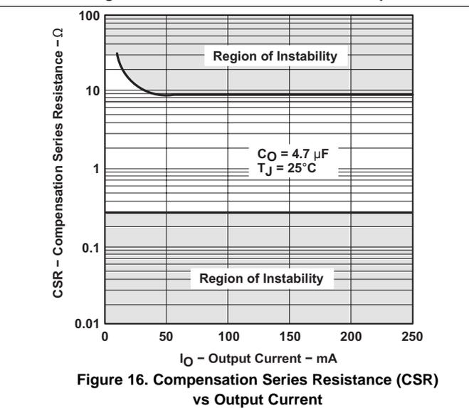
Figure 16. Compensation Series Resistance (CSR) vs Output Current
