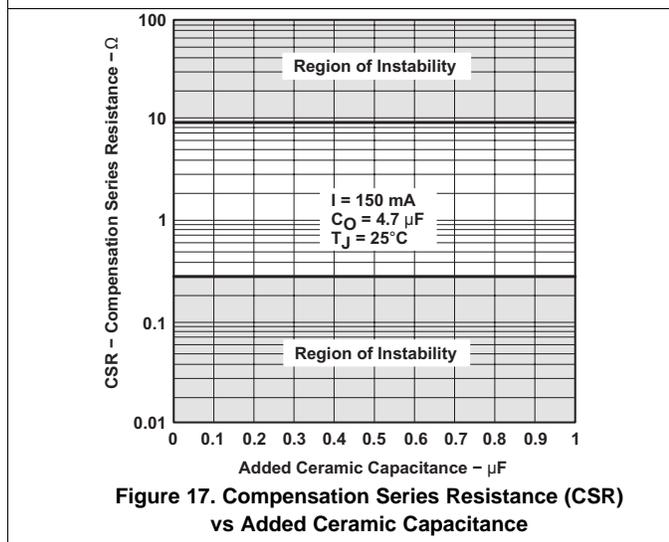
Figure 17. Compensation Series Resistance (CSR) vs Added Ceramic Capacitance
