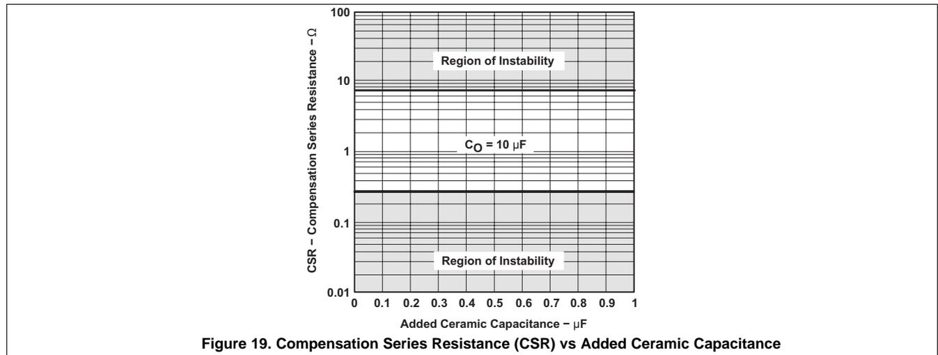
**Figure 19. Compensation Series Resistance (CSR) vs Added Ceramic Capacitance**
