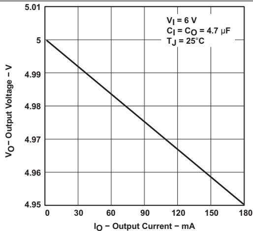
Figure 3. TPS76350 Output Voltage vs Output Current
