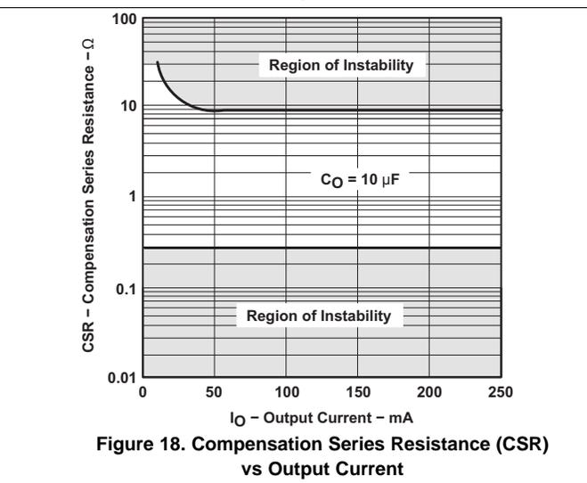
Figure 18. Compensation Series Resistance (CSR) vs Output Current
