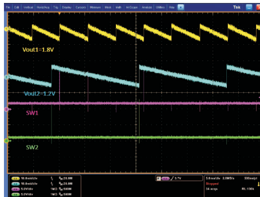
Figure 12. Buck 1 and Buck 2 in PSM Mode
