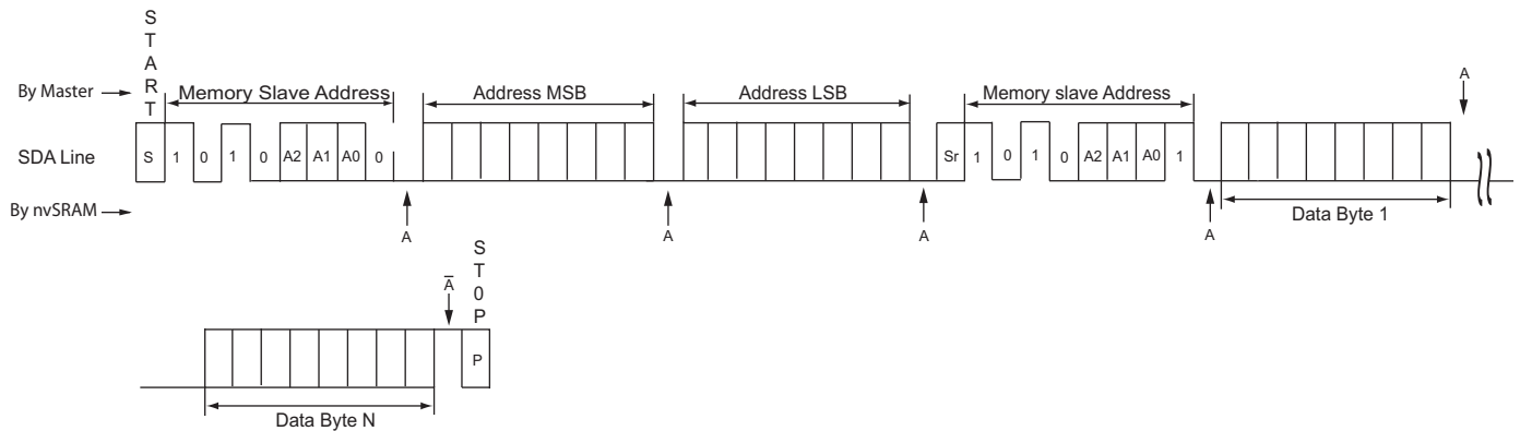
Figure 21. Random Address Single-Byte Read (Hs-mode)
