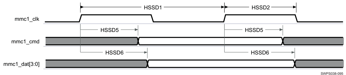
Figure 6-66. MMC1 Interface—High-Speed SD Mode—Data/Command Transmit
