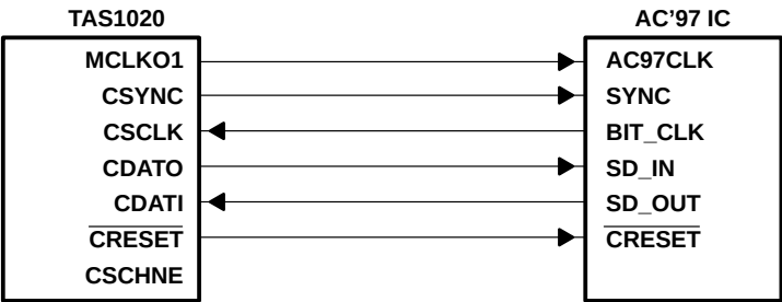
Figure 2–2. Connection of the TAS1020 to an AC '97 Codec
