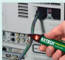
Locate power cord breaks
