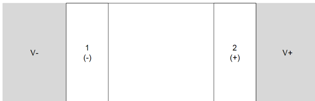
Figure 22. DEC Package Recommended Layout
