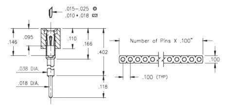
**Description:** Interconnect Socket Elevated Strip Socket Accepts .015" - .025" (0,38 - 0,635 mm) dia leads Single Row Through Hole Plating Code: **Shell Plating:**
