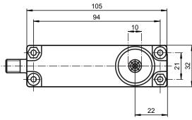
Bore hole and countersinking for screws/hexagon M4
