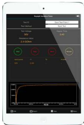
Figure 2. Perform remote testing with Keysight InsulationTester Application
