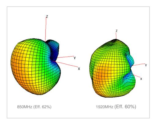
Note: The 3D Gain pattern and efficiency shown above is as measured with the antenna mounted on a particular GE meter at 3'O Clock position.
