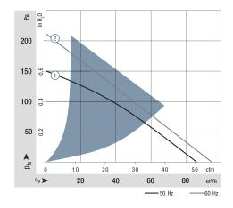
Air performance measured according to: ISO 5801. Installation category A, without contact protection. Noise: Total sound power level  $L_WA$  ISO 103002 measured on a hemisphere with a radius of 2 m. Sound pressure level LpA measured at 1 m distance
