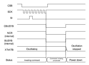
The regulator and the speaker amplifier stop operation after a lapse of command processing time after the PDWN command is input. At this time, the SPM output of the speaker amplifier goes to a Hi-Z state to prevent troubles by pop noise.
