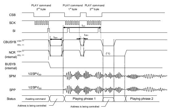
\*1: The time length of "L" level of the NCR signal during playback varies depending on the input timing of command.
