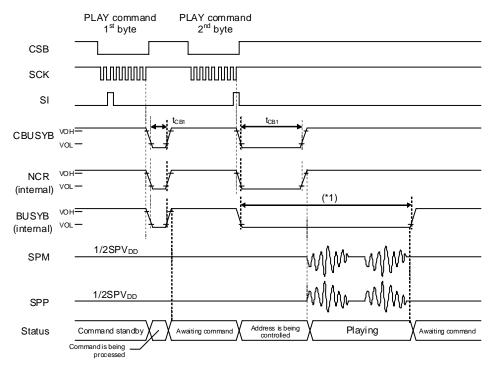
Note: The length of the "L" interval of BUSYB is  $t_{\text{CB1}}$  + voice reproduction time.
