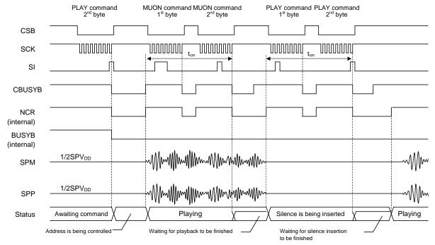
When the playback starts after the PLAY command is input and the address control of phrase-1 is over, the CBUSYB and NCR signals go to "H" level. Input the MUON command after this CBUSYB signal changes to "H" level. After the MUON command input, the NCR signal remains at "L" level until the end of phrase-1 playback. This status is the waiting for the phrase-1 playback to be finished.
