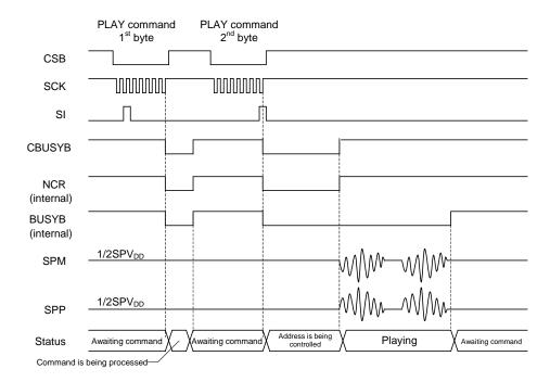
When the 1<sup>st</sup> byte of the PLAY command is input, the device enters a state awaiting input of the 2<sup>nd</sup> byte of the PLAY command after a lapse of command processing time.
