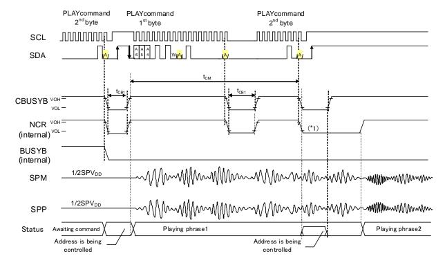
\*1: The time length of "L" level of the NCR signal during playback varies depending on the input timing of command.
