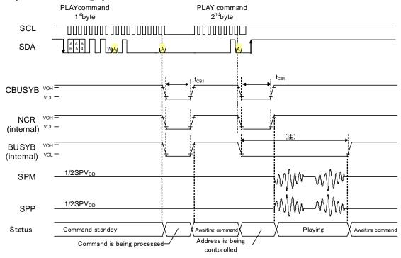
Note: The length of the "L" interval of BUSYB is  $t_{\text{CB1}}$  + voice reproduction time.
