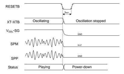
Note: The same timing is applied in the case that the RESETB signal is input during command waiting.
