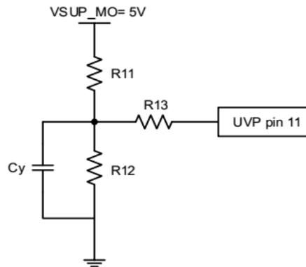
$V_{UVP} = (1.21V - 4.7\mu A * R13) * (R11 + R12) / R12$ ;  $V_{hysteresis} = 4.7\mu A * R13 * (R11 + R12) / R12$ ; With the condition  $R13 \gg R11 // R12$ . For example, if  $R11 = 5.6k$ ,  $R12 = 2.2k$  and  $R13 = 47k$ , then  $V_{UVP} = 3.506V$ ;  $V_{hysteresis} = 0.783V$ . Here,  $V_{UVP}$  is the shut down threshold. In this case, the voltage at UVP pin 11 is greater than 1.431V under worst case of VSUP\_MO ripples.
