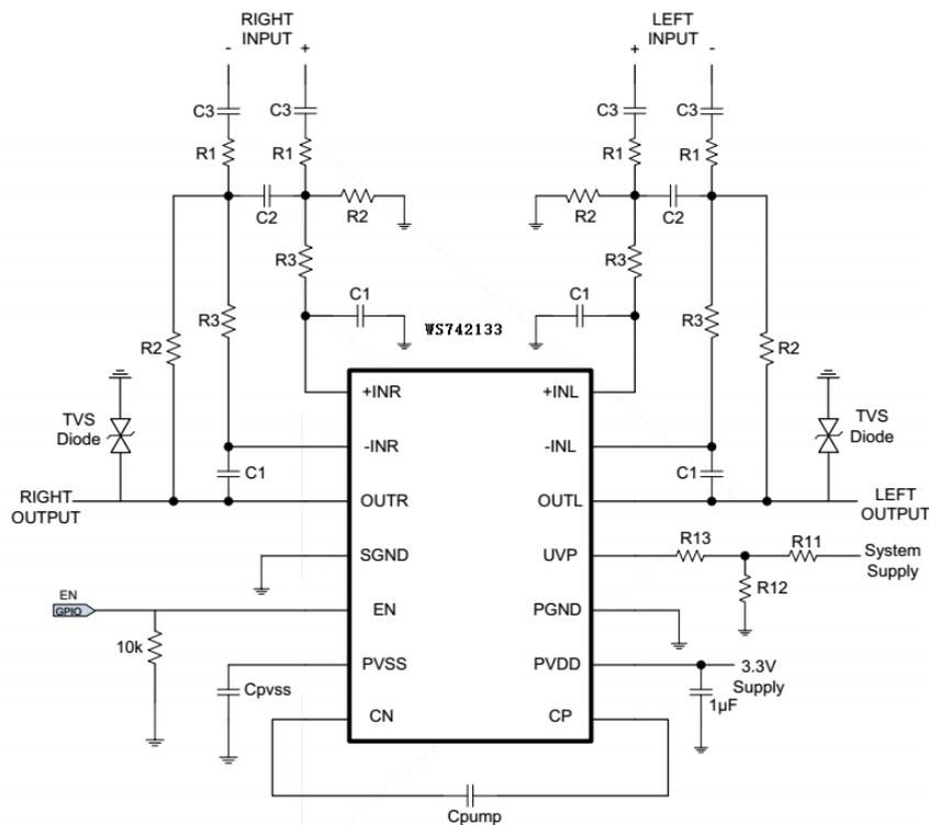
Differential-input, single-ended output, second-order filter R1=15kΩ, R2=30kΩ, R3=47kΩ, C1=33pF, C2=150pF, C3=6.8µF, R11=5.6kΩ, R12=2.43kΩ, R13=15KΩ, Cpvss=0.33 to 1µF, Cpump=0.33 to 1µF.
