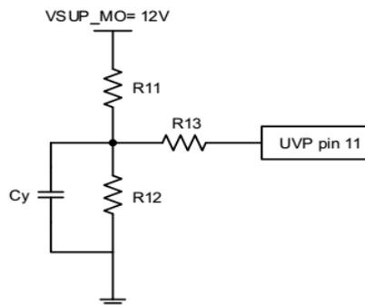
$V_{UVP} = (1.21V - 4.7\mu A * R13) * (R11 + R12) / R12$ ;  $V_{hysteresis} = 4.7\mu A * R13 * (R11 + R12) / R12$ ; With the condition  $R13 \gg R11 / R12$ . For example, if  $R11 = 11k$ ,  $R12 = 1.4k$  and  $R13 = 47k$ , then  $V_{UVP} = 8.76V$ ;  $V_{hysteresis} = 1.957V$ . Here,  $V_{UVP}$  is the shut down threshold. In this case, the voltage at UVP pin 11 is greater than 1.431V under worst case of VSUP\_MO ripples.
