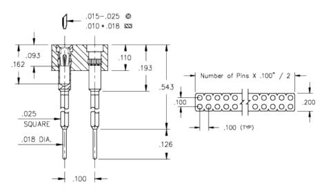
**Description:** Interconnect Socket Wrapost with Solder Tail Socket Accepts .015"- .025" (0,38 - 0,635 mm) dia leads Double Row Through Hole Plating Code:
