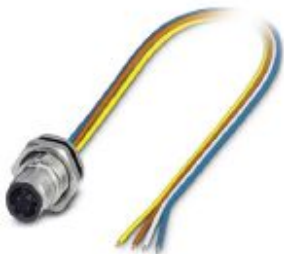
Bus system flat-type plug, 4-position, Plug, M12, D-coded, Rear mounting, M16 x 1.5, Individual wires, cable length: 0.5 m, 0.34 mm 2 , TPE litz wire
