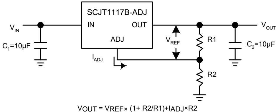
The output voltage of adjustable version follows the equation:  $V_{out} = 1.25 \times (1 + R2/R1) + I_{Adj} \times R2$ . We can ignore  $I_{Adj}$  because  $I_{Adj}$  (about 50µA) is much less than the current of  $R1$  (about 2~10mA).
