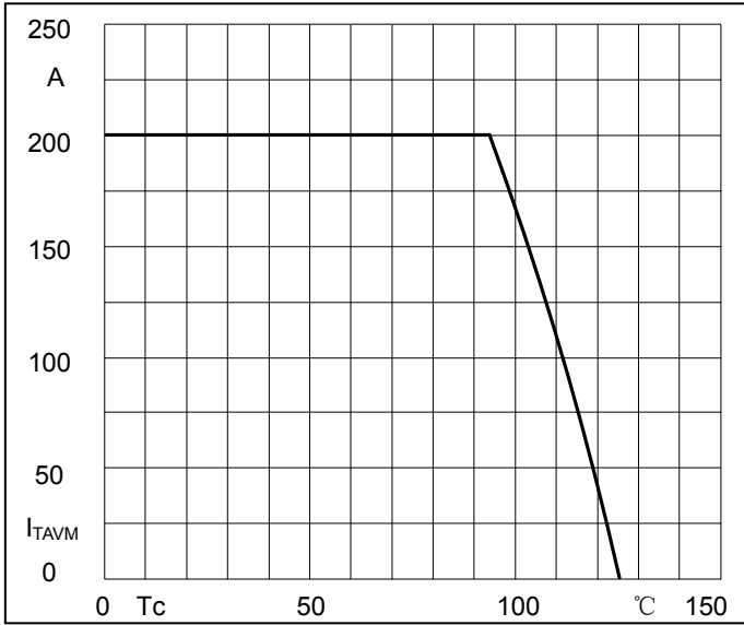
Fig7. SCR Forward Current Derating Curve
