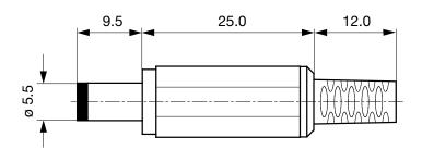
Cable diameter max. 4.0 mm
