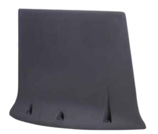
The Harris RF-7850A-AT002 is a vertically polarized, omni-directional UHF antenna operating within the 225-512 MHz frequency range. Designed for use with the Harris RF-7850A Falcon III® Airborne Networking radios, the AT002 is ruggedized for reliability during use on helicopters and subsonic aircraft. This antenna handles up to 150 watts of power, does not require external tuning and is DC grounded to drain static charges.
