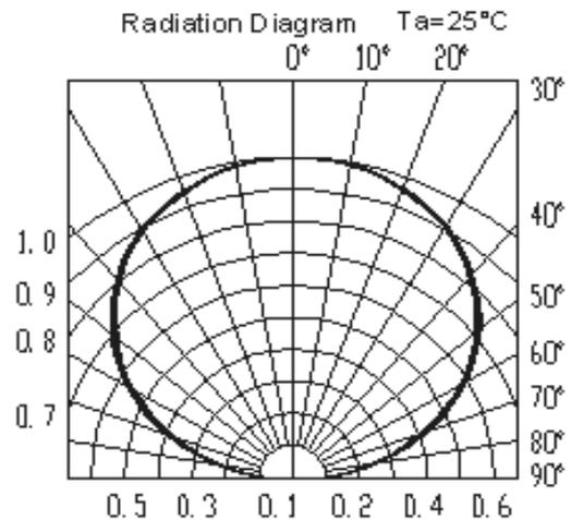
Typical Electro-Optical Characteristics Curves
