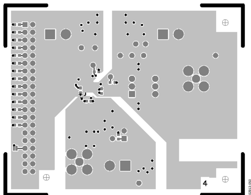
Figure 53. LFCSP Evaluation Board Layout—Secondary Side
