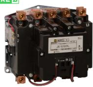
NEMA Contactor, Type S, nonreversing, Size 4, 135A, 100 HP at 575 VAC, 3 phase, up to 100 kA, 5 pole, 480 VAC coil, open
