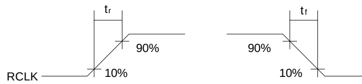
Fig. 12 Signal Rise and Fall Characteristics
