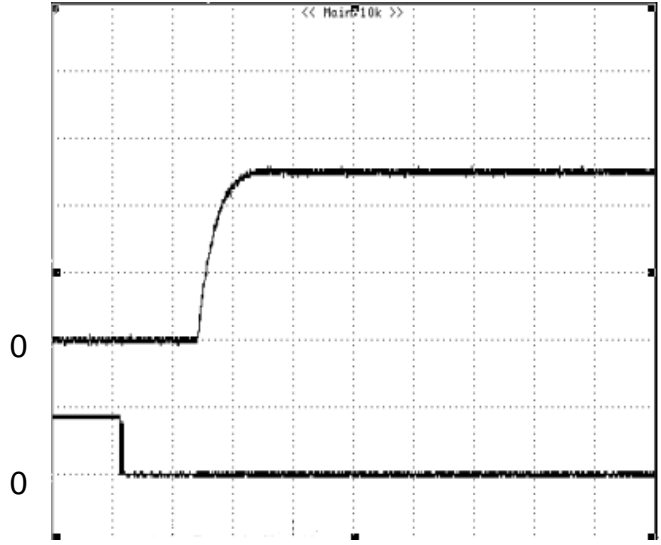
Figure 5: Turn-on transient at zero load current (1 ms/div). V_{in}=48V . Top Trace: V_{out} , 1.0V/div; Bottom Trace: ON/OFF input, 5V/div
