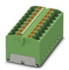
Distribution block, bridged internally, nom. voltage: 450 V, nominal current: 32 A, connection method: Push-in connection, number of connections: 18, cross section: 0.2 mm² - 6 mm², AWG: 24 - 10, width: 55.4 mm, height: 21.7 mm, color: green, mounting type: for snapping onto a DIN rail adapter, for snapping onto a DIN rail adapter, Adapter plate, Adapter plate
