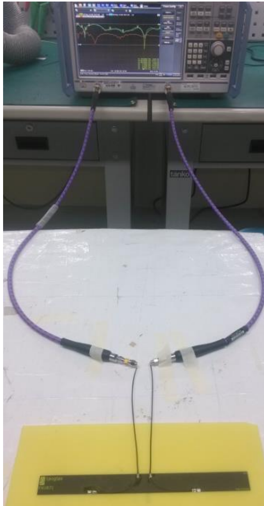
Figure.1 Test setup on the 2mm ABS
