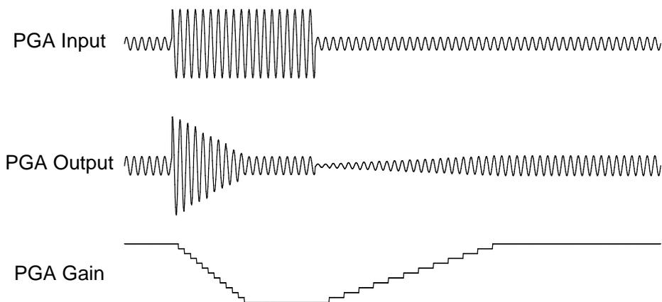
Figure 7: ALC Normal Mode Operation
