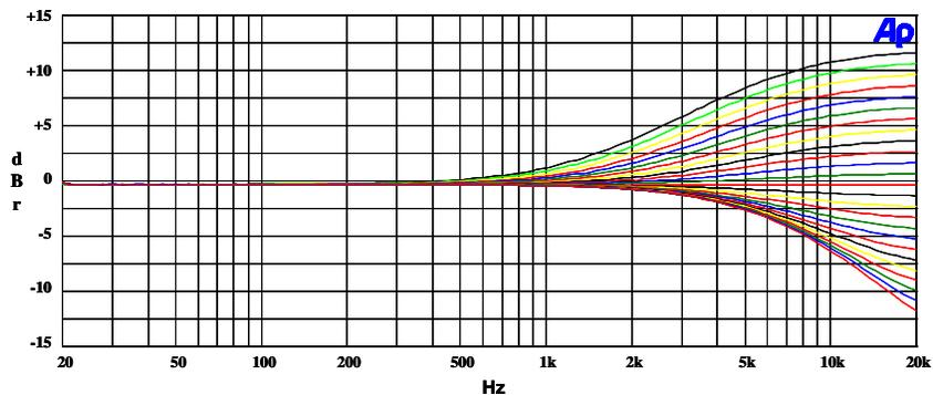
Figure 52: EQ Band 5 Gains for Lowest Cut-Off Frequency
