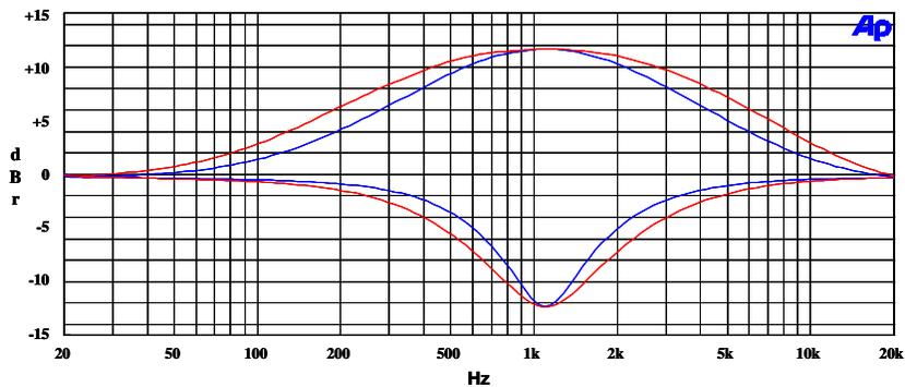
Figure 49: EQ Band 3, EQ3BW = 0 versus EQ3BW = 1
