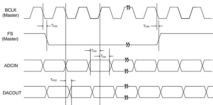
Figure 34: Digital Audio Interface Master Mode Timing
