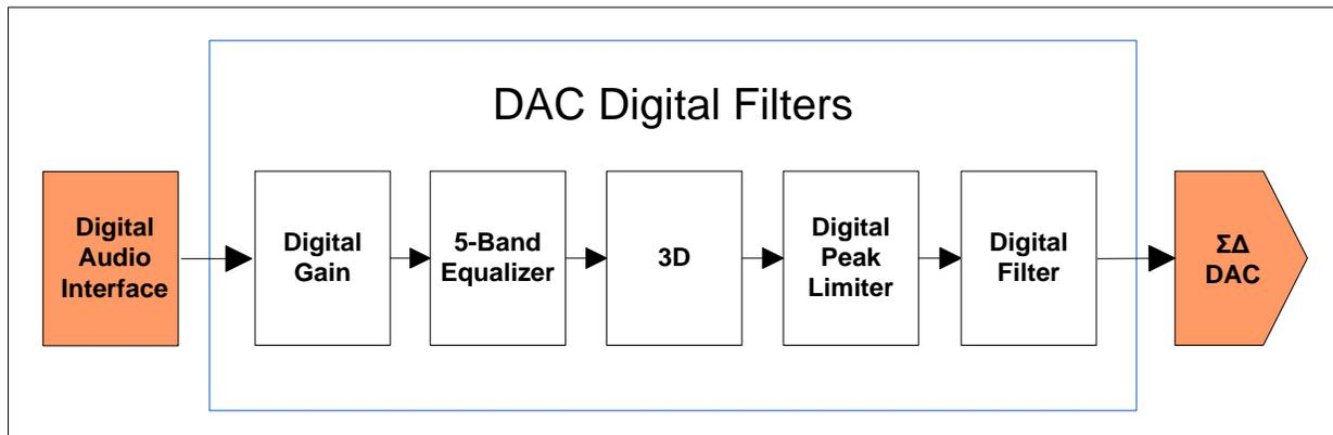
The DAC digital block uses 24-bit signal processing to generate analog audio with a 16-bit digital sample stream input. This block consists of a sigma-delta modulator, digital decimator/filter, and optional 5-band graphic equalizer/3D effects block, and a dynamic range compressor/limiter. The DAC coding scheme is in twos complement format and the full-scale output level is proportional to  $V_{DDA}$ . With a 3.3V supply voltage, the full-scale output level is  $1.0V_{RMS}$ .
