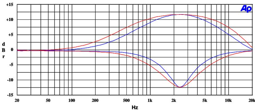
Figure 51: EQ Band 4, EQ4BW = 0 versus EQ4BW = 1
