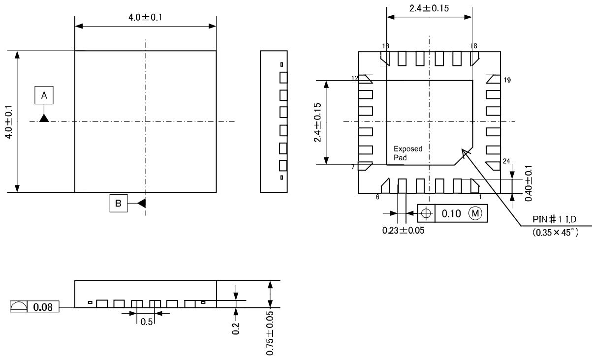
**Note** The exposed pad at the center of the back of the package must be connected to VSS or opened.
