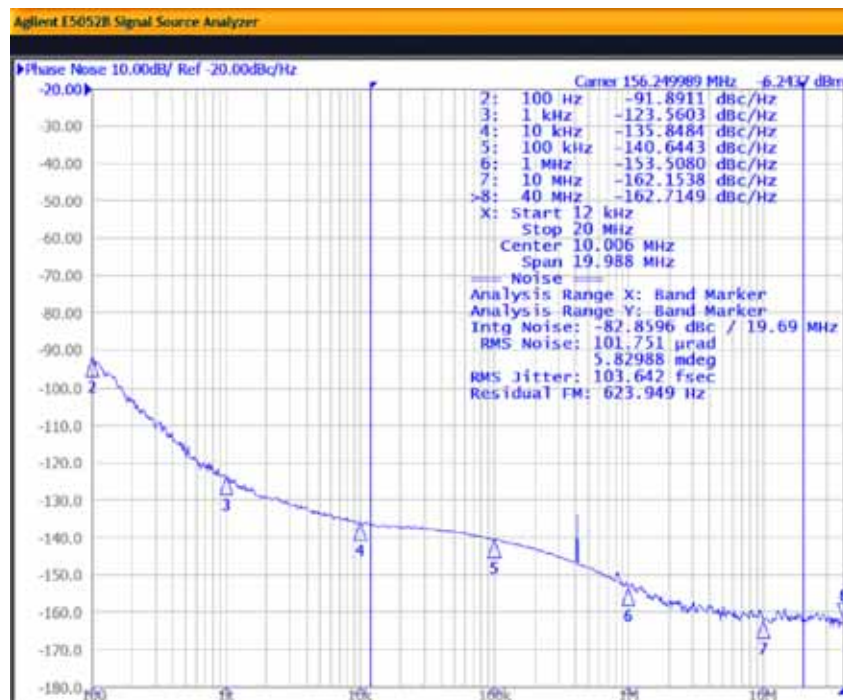
Figure 6. Input = 25 MHz; Output = 156.25 MHz, 2.5 V LVDS
