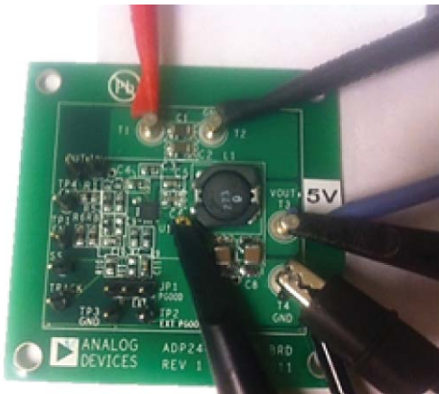
Figure 4. Switch Node Measurement
