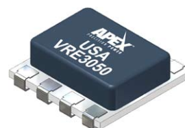
8-pin Surface Mount Package Style GF
