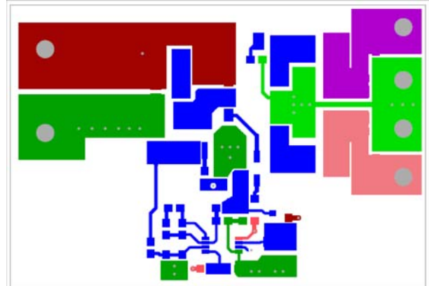
FIGURE 2. ISL6844EVAL3Z - TOP LAYER (COMPONENT SIDE)
