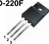
1.Gate 2. Drain 3. Source
