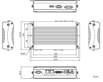
When you fasten the bundled attachment fittings to be fixed to the body, you should use the attached screws (M4 x 10). Otherwise, the length (L) from the surface of the cabinet to the screw tip should be 5mm or less.
