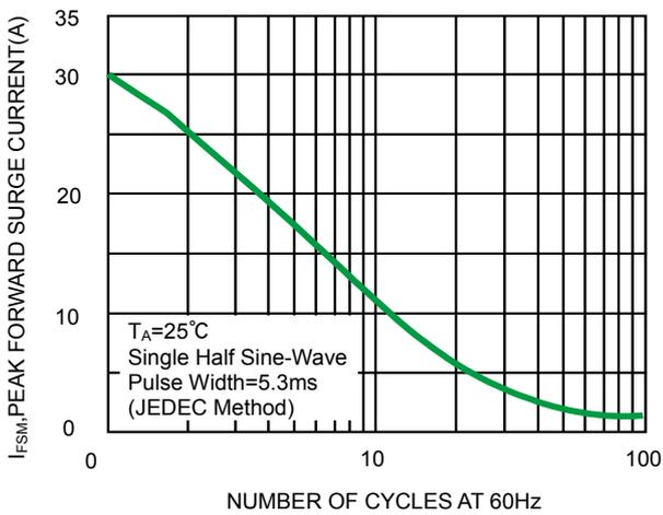
Fig 3. Maximum Peak Forward Surge Current(per leg)
