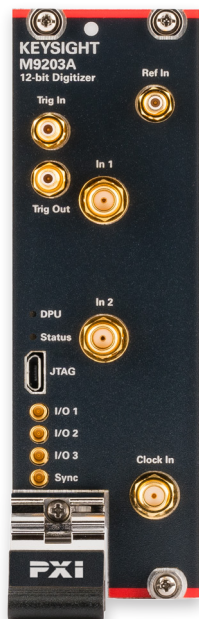
Figure 3. M9203A front panel with analog inputs and multiple I/O signals.
