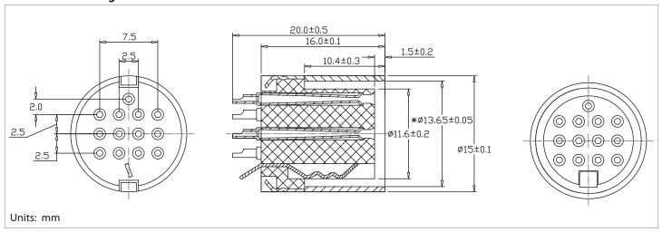
tolerance X:  $\pm 0.5 \, \text{mm}$  .X:  $\pm 0.3 \, \text{mm}$  .XX:  $\pm 0.05 \, \text{mm}$  applicable unless otherwise indicated in specification or on drawings
