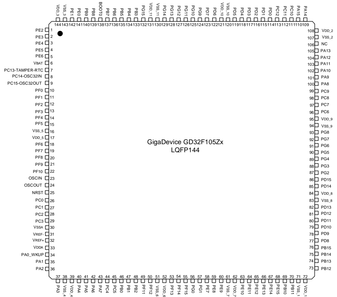
Figure 2-2. GD32F105Zx LQFP144 pinouts
