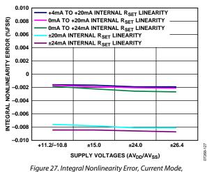
Internal R<sub>SET</sub> Sense Resistor
