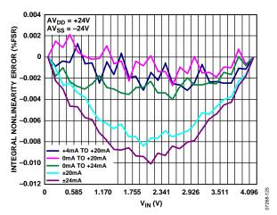
Figure 25. Integral Nonlinearity Error vs. V<sub>IN</sub>, Internal R<sub>SET</sub> Resistor
