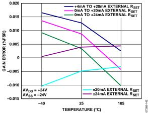
Figure 42. Gain Error vs. Temperature, External R<sub>SET</sub> Sense Resistor
