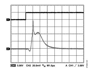
Figure 20.  $V_{OUT}$  Enable Glitch, Load = 2 k $\Omega \parallel 1 nF$
