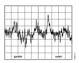
Figure 21. Peak-to-Peak Noise (0.1 Hz to 10 Hz Bandwidth)
