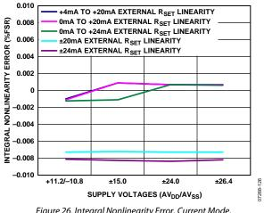
Figure 26. Integral Nonlinearity Error, Current Mode, External R<sub>SET</sub> Sense Resistor
