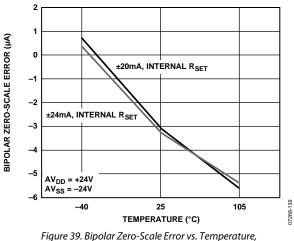
Internal R<sub>SET</sub> Sense Resistor
