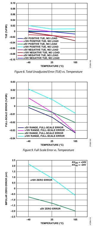
Figure 10. Bipolar Zero Error vs. Temperature
