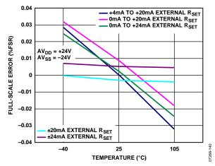
Figure 40. Full-Scale Error vs. Temperature, External R<sub>SET</sub> Sense Resistor
