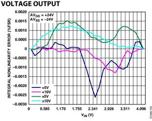
Figure 5. Integral Nonlinearity Error vs. VIN
