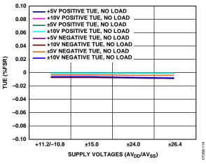
Figure 14. Total Unadjusted Error (TUE) vs. Supply Voltages
