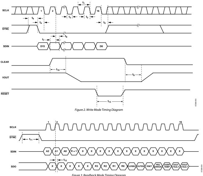
Figure 3. Readback Mode Timing Diagram
