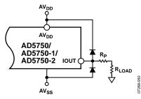
Figure 56. Output Transient Voltage Protection
