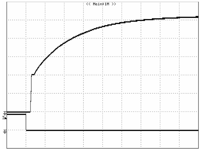
Figure 5: Turn-on transient at zero load current (5 ms/div). Top Trace: Vout: 10V/div; Bottom Trace: ON/OFF input: 5V/div.
