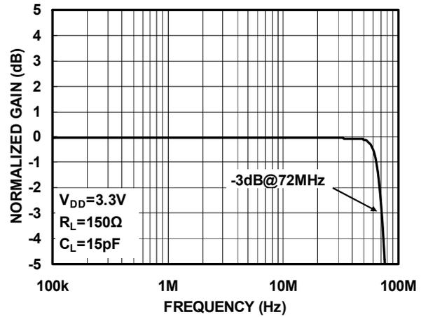
Figure4. Large-Scale Frequency Response
