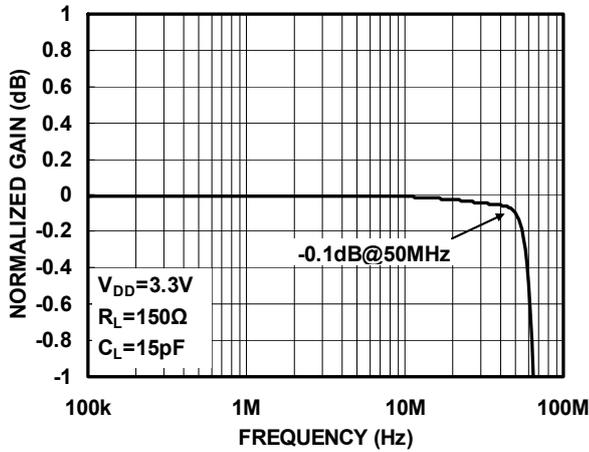
Figure3. Small-Scale Frequency Response
