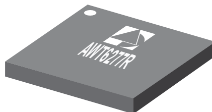
M20 Package 10 Pin 4 mm x 4 mm x 1.1 mm Surface Mount Module
